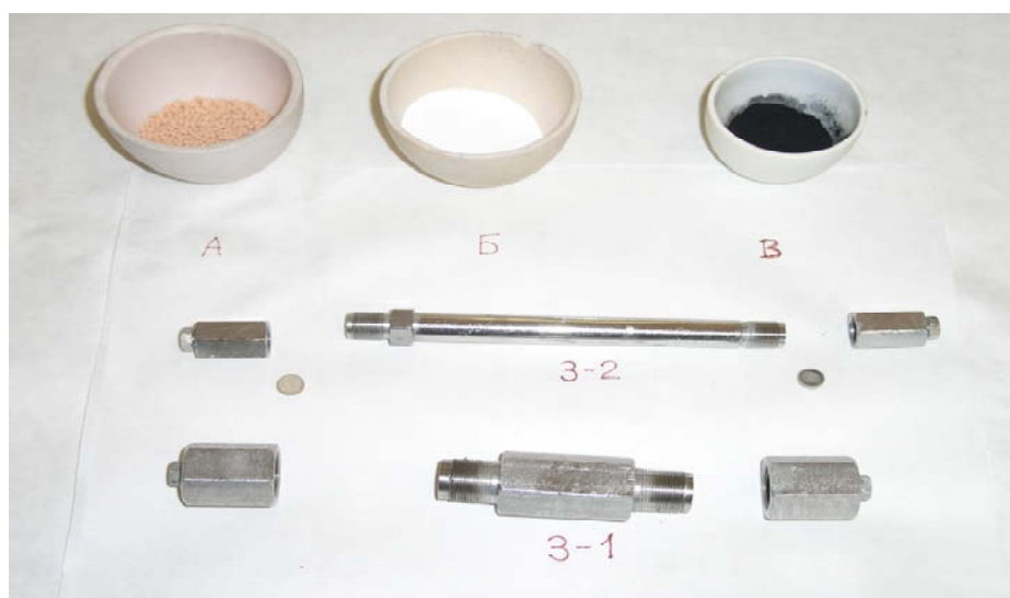
Fig. 3. Cells for radionuclides 3.1 (10.5 ml) and for sorbent 3-2 (10.2 ml) and sorbents: A – zeolite NaA, Б – silica gel Silochrom II, B – activated carbon.
